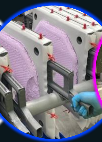
Mixed Rare Earth Oxide cake from filter press
